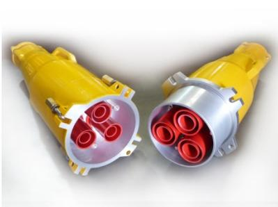
Couplers rated up to 15kV, 500A are used to power large pit equipment. This system is similar to the design of the IMG 8kV couplers and incorporates many of the same features: 3 piece insulators; interlock system, LLI, body bars, entrance fitting, and such. The IMG entrance fitting used in these couplers fits the 8, 15 & 25kV coupler range. The entrance fitting is completely moisture-proof thus eliminating the need for body filling.
