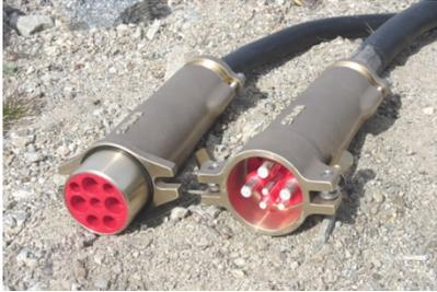
1.1kV couplers are typically used in hard-rock mining or tunnelling operations. They are used to distribute power to electrical site equipment such as shovels, drillers, pumps, controllers, motors & such. Couplers are available in: 170A or 250A rating; Aluminum or Bronze housing; powder-coated or bare metal; 1 or 2 Control/Pilot Pins; Cable-mount or Equipment-mount style
